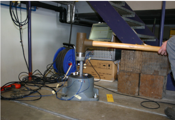
Fig.1.7 Vibro-Acoustic Transfer Function measured across Propeller bearing
